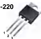
1.Gate 2. Drain 3. Source
